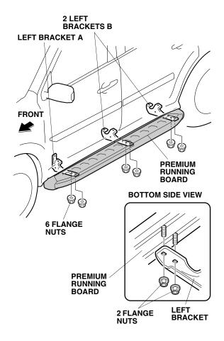
6. Align the center of the premium running board as shown.
