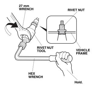
Remove the rivet nut tool from the rivet nut by turning the hex wrench counterclockwise.  Install left bracket A on the vehicle frame with two flange bolts. Do not tighten the flange bolts yet.
