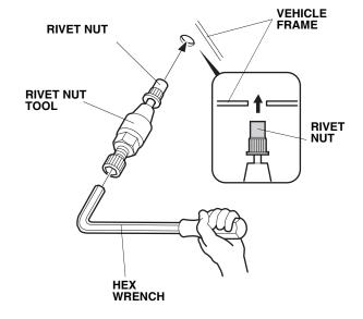
Holding the rivet nut tool with the hex wrench, turn the 27 mm wrench clockwise and install the rivet nut in the vehicle frame.
