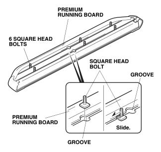
5. Position the premium running board on the left bracket A and the two left brackets B. Install the premium running board with six flange nuts. Do not tighten the flange nuts yet.
