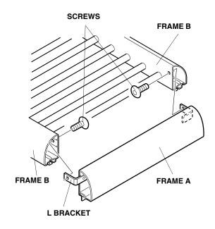
6. Install the remaining frame A to the frames B in the same way.
