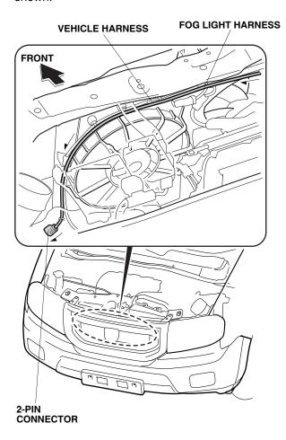
14. Route the fog light harness 2-pin connector to the underside of the vehicle.
