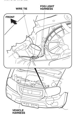
18. Secure the fog light harness to the vehicle harness with five wire ties.
