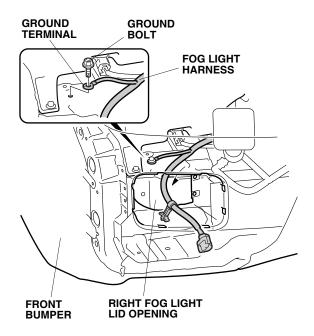
Pull the fog light harness 2-pin connector (shorter section of the harness) out of the right fog light lid opening.
