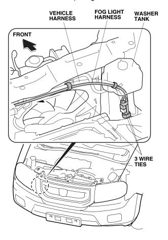
12. Secure the fog light harness to the vehicle harness with three wire ties.
