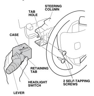
32. Install the new headlight switch on the steering column using the two self-tapping screws. Hold the case by hand, then install the new headlight switch to the steering column. Do not push on the lever when installing the case. Push on the case only and set the retaining tab to the tab hole securely.
