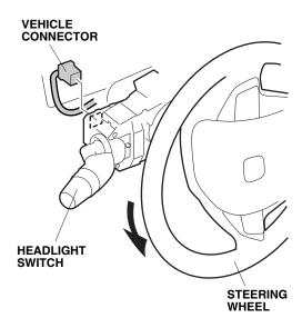
31. Remove the two self-tapping screws from the headlight switch. While pushing the retaining tab, slide the headlight switch, and remove it from the steering column. Do not pull on the lever when removing the case. Do not damage the tab hole in the steering column.
