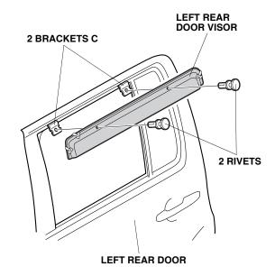
15. Adjust the position of the left rear door visor. Make sure that there is no clearance between the bracket and the door sash.
