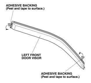
4. Using isopropyl alcohol on a shop towel, clean the door sash where the left front door visor will attach.
