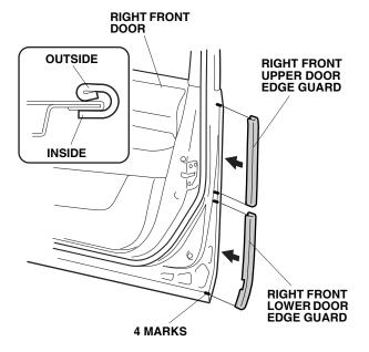
Make sure they are positioned correctly, then tap the right front door edge guards into position with a series of light taps with a rubber mallet. Once in place, do not remove, reposition, or reinstall the right front door edge guards or they will not hold securely.
