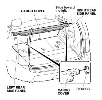
5. Pull out the cargo cover, and attach the right and left hooks of the cargo cover to the right and left rear side panel.
