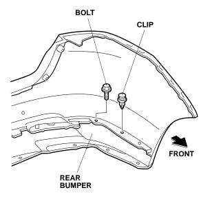
10. Align the hole in the template with the bolt and clip holes, and tape template B (large portion) to the bumper.
