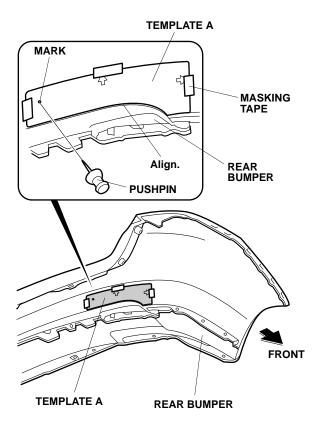
3. Using a pushpin, pierce a hole through the bumper at the mark on the template. Remove the template.
