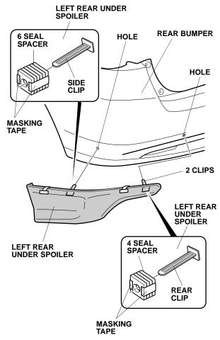
20. Install one six seal spacer over the side clip, install one four seal spacer over the rear clip, and install the left under spoiler to the bumper.
