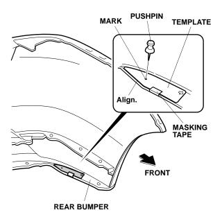
6. Using a pushpin, pierce a hole through the bumper at the mark in the template. Remove the template.
