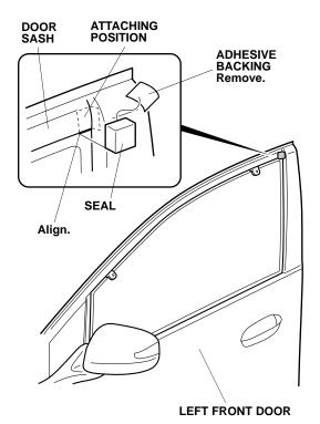
6. Peel back approximately 1-1½ inches of adhesive backing from each adhesive tape, and tape the ends to the front surface of the left front door visor.
