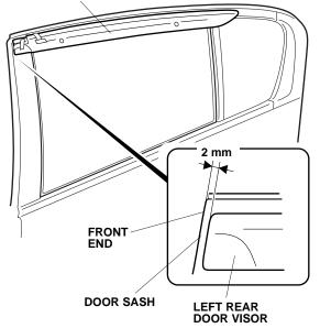
19. While holding the door visor up firmly, remove the adhesive backing. Use your finger to push up each bracket so there is no gap between the brackets and the door sash.
