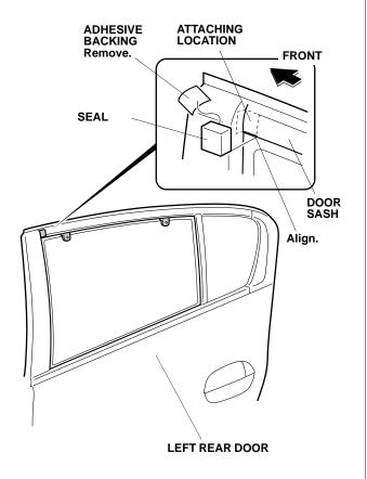
16. Peel back approximately 1-1½ inches of adhesive backing from each adhesive tape, and tape the ends to the front surface of the left rear door visor.
