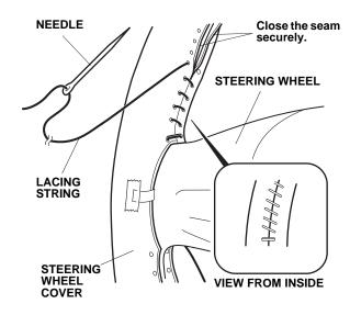
8. Keep stitching while adjusting the steering wheel cover so the joints on the cover are aligned.
