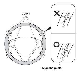
9. Stitch the spoke area of the steering wheel cover as shown. Stitch twice at the holes in the steering wheel cover that are right below and right above the spoke.
