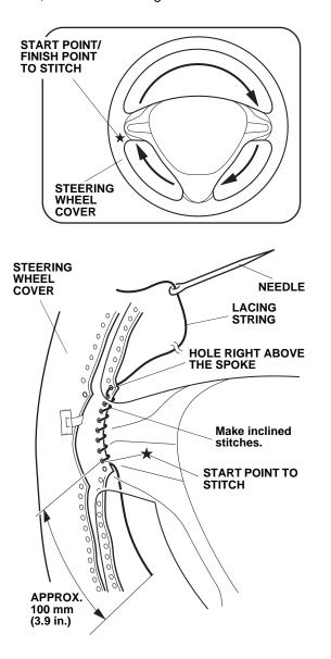
6. Stitch twice through the holes right above the spoke, and pull the lacing string to close the seam securely.
