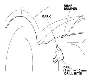
While wearing eye protection, drill a 10 mm hole through the left rear splash guard. First drill with a 3 mm drill bit, then finish with a 10 mm drill bit. Remove all burrs.
