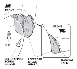
12. Using a pushpin, pierce the rear bumper at the mark through the left rear splash guard.
