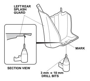
16. Install the left rear splash guard using the one self-tapping screw that you removed and two clips. Tighten the self-tapping screw and install the clips in the order shown below while pushing the left rear splash guard against the vehicle body.
