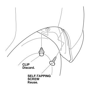
11. With the vehicle on a lift, temporarily install the left rear splash guard using one clip, the self-tapping screw from step 10, and a strip of masking tape. Make sure there is no gap between the left rear splash guard and the vehicle.
