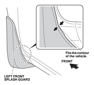
7. While pushing the left front splash guard firmly against the vehicle body, tighten the self-tapping screws securely in the order shown below. Make sure there is no gap between the left front splash guard and the vehicle.
