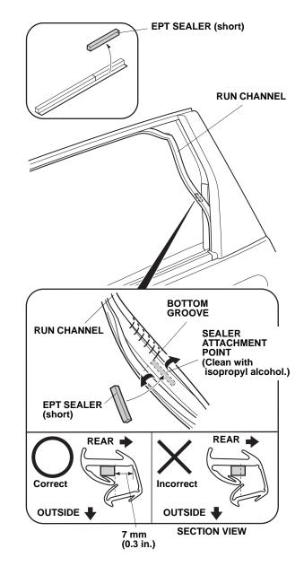
10. Remove an EPT sealer (short) from the adhesive backing, and attach it as shown. Make sure it is attached securely.
