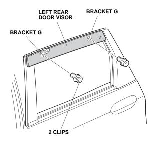
19. Push the left rear door visor upward, and check that it aligns with the contour of the door sash. Push the brackets firmly against the door sash so there is no gap between the clips and the sash.
