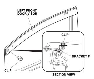
34. Secure the left front door visor to the bracket F with a clip.
