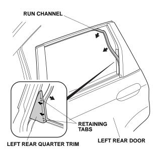
8. Pull out the rear corner of the run channel.
