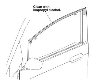
29. Remove the adhesive backing from a sealer, and attach it to the left front door as shown.
