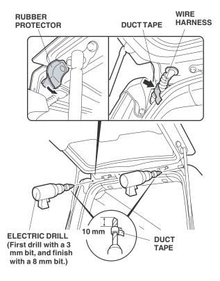
Temporary install the tailgate spoiler on the tailgate and insert the two bolts into the 8 mm holes. Using a felt-tip pen, mark the tailgate through the center hole in the tailgate spoiler. Remove the tailgate spoiler, being careful not to drop any bolts on the vehicle.
