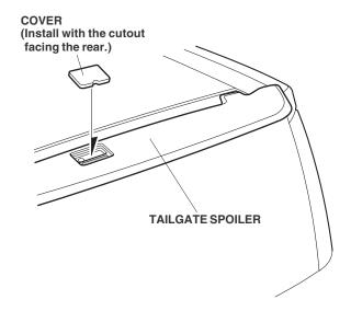
20. Press down and hold the tailgate spoiler at the adhesive tapes for 30 seconds.
