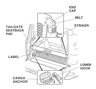
2. Attach the tailgate seat back pad lower hooks to the left and right cargo anchors on the vehicle.
