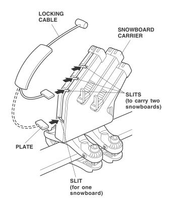
15. After loading the snowboard(s) on the carrier, adjust it (them) with the help of the board supports so that the top edges are level and the boards are as far down in the carrier as possible. To secure the snowboard(s) use the key to open the covers, and insert the locking cable stops into the holes of the carrier covers.
