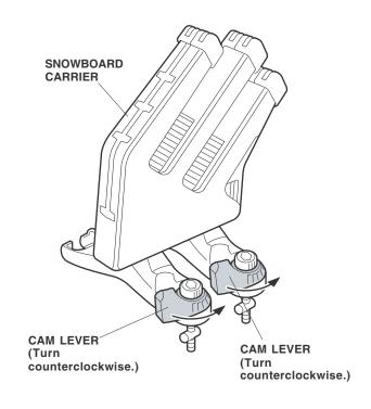
5. Attach the two bottom clamps to the two top clamps.
