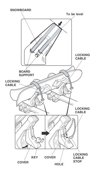
16. Check that the locking cables are installed securely, then close the covers.
