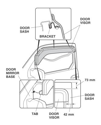
Adjust the location of the door visor so that the clearance between the door visor and door sash is 73 mm at the top, and 42 mm at the back. There should be no clearance between the door mirror base and the visor.
