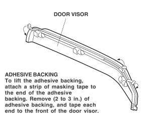
4. Insert the front tab of the door visor under the door mirror base, and attach the three brackets to the door sash.
