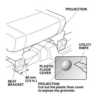
2. Install a front floor mat anchor to each of the three grommets using one self-tapping screw for each floor mat anchor.
