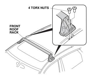
24. Repeat steps 22 and 23 to remove the rear roof rack.
