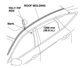
2. Using a plastic trim tool, pry up the edge of the roof molding in the areas shown.
