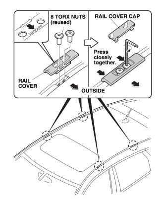
26. Snap the rail cover cap onto the rail cover. Pull the rail cover outward, and align the cover with the roof molding.
