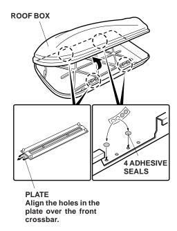
Attach adhesive seals over the unused rear mounting holes along the bottom of the roof box.
