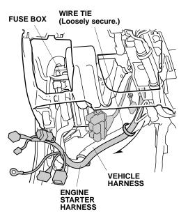
40. Using one wire tie, loosely secure the engine starter harness to the vehicle harness.
