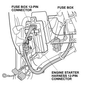
NOTE: If another accessory 12-pin connector is already plugged into the fuse box: Unplug the 12-pin connector from the fuse box, then plug the engine starter harness 12-pin connector into the fuse box. Remove and discard the dummy connector from the engine starter harness, and plug the other accessory 12-pin connector into the engine starter harness 12-pin connector.
