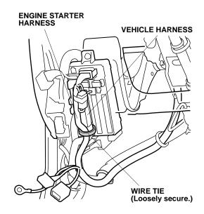
44. Unplug the vehicle 20-pin connector (blue), and plug it into the engine starter harness 20-pin connector. Plug the engine starter harness 20-pin connector (white) into the vehicle 20-pin connector.
