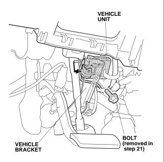
39. Route the engine starter harness along the vehicle harness to the front of the fuse box.
