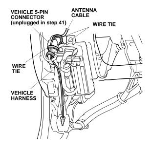
64. Using two wire ties, secure the antenna cable to the vehicle harness.
