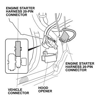
46. Remove and discard the hood opener bolt. Install the ground bolt with the engine starter harness ground terminal attached.
