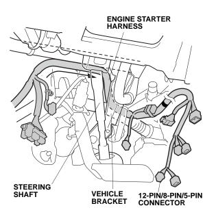
27. Route the 12-pin/8-pin/5-pin connector end of the engine starter harness to the ignition switch.
