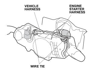
Using two wire ties, secure the engine starter harness to the vehicle harness in the areas shown.
