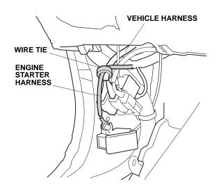
48. Using two wire ties, loosely secure the engine starter harness to the vehicle harness.
