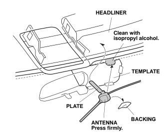
56. Remove the backing from the antenna. Insert the antenna plate under the headliner, align the antenna with the template, and attach the antenna to the windshield. Press the antenna firmly.
