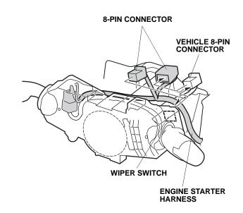
32. Using two wire ties, secure the engine starter harness to the vehicle harness. Do not secure it to the SRS harness.
