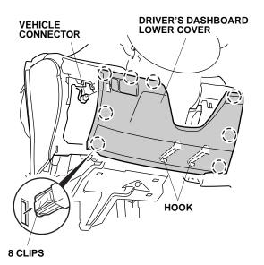
13. Remove the driver's dashboard under cover (three clips and one pin).
