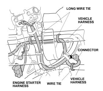
37. Using two long wire ties, secure the engine starter harness to the vehicle harness at the locations shown.
