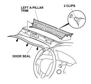
11. Remove and discard the clip from the left A-pillar trim, and install a new A-pillar clip (supplied) onto the left A-pillar trim.
