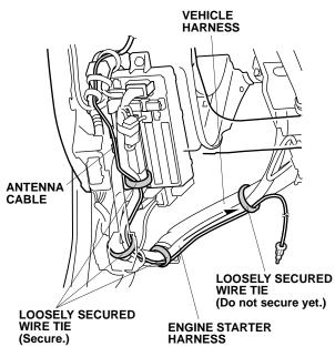
66. Secure the antenna cable using the three loosely secured wire ties.
