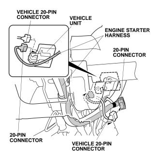
35. Align the green tape on the engine starter harness with the clip on the vehicle harness, and secure the engine starter harness to the vehicle harness using one wire tie.
