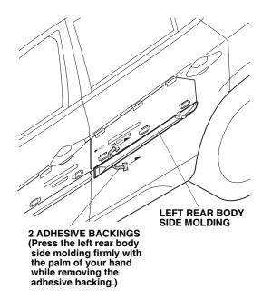
Using the rubber roller, apply firm pressure while rolling to set the adhesive. Apply firm pressure especially at the ends.
