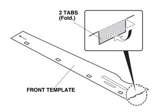
2. Insert the two tabs on the front template around the rear edge of the left front door.
