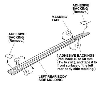
13. Align the edges of the left rear body side molding with the edges of the rear template, and install the left rear body side molding on the left rear door.
