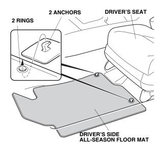
**4WD model:** Place the grommets in the driver's side all-season floor mat over the tabs, and turn the tabs one quarter turn to secure the all-season floor mat.
