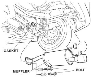
Torque the bolts to 22 N·m (16 lb-ft), alternating 4. from side to side.
