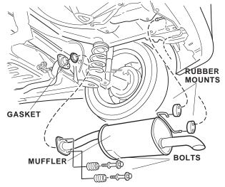
Remove the old exhaust gasket, and replace it with the new exhaust gasket from the kit.
