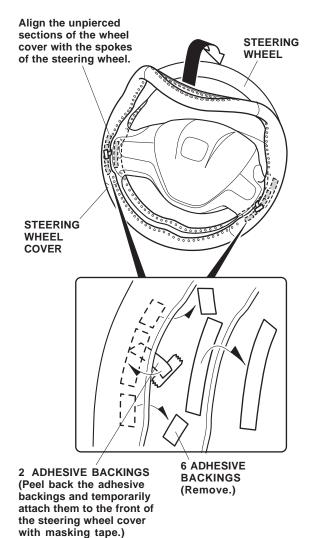
Pull back the steering wheel cover. Peel back the adhesive backings shown, and temporarily attach them to the front of the steering wheel cover with masking tape. Remove all the remaining adhesive backings from the steering wheel cover.
