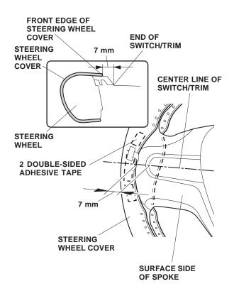
Align the rear edge of the steering wheel cover to the back of the steering wheel spoke as shown.
