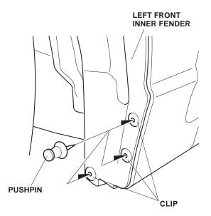
Position the left front splash guard on the left front 3. inner fender, and install the three 5 x 20 mm selftapping screws. Tighten the three self-tapping screws in the order shown.
