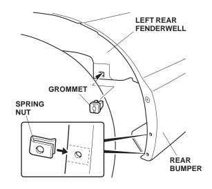
Position the left rear splash guard on the left rear 7. fenderwell and rear bumper, then install the two 5 x 25 mm self-tapping screws and one 5 x 20 mm self-tapping screw. Tighten the three self-tapping screws in the order shown cut off any excessive under coat material with a utility knife.
