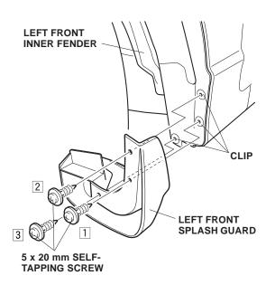
Turn the steering wheel all the way clockwise, 4. and repeat steps 2 and 3 to install the right front splash guard.
