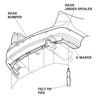
NOTE: If a gap is visible between the rear bumper and under spoiler, remove the under spoiler and confirm the location of the marks with a tape measure. If necessary, create new marks in the proper locations.
