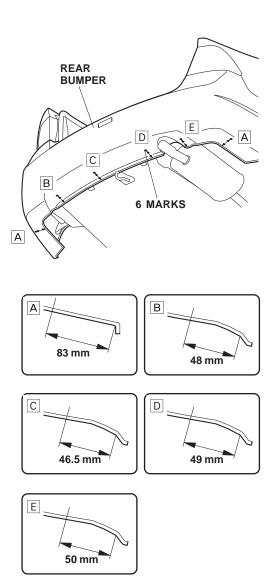
9. Using a pushpin, make a hole through each marked location on the rear bumper.
