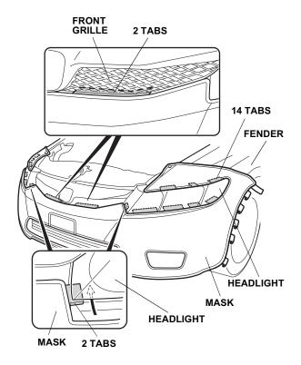
9. Pull the mask toward the wheelwell, smooth out any wrinkles, and attach the five plastic hooks to the fenderwell, then bend the metal tab around the fenderwell. Repeat on the other side.
