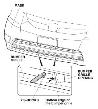
13. Route the elastic cord through the ten loops on the bottom of the mask. Attach one S-hook to the bottom edge of the bumper on one side. Stretch the cord, then attach the other S-hook to the bottom edge of the bumper on the other side.
