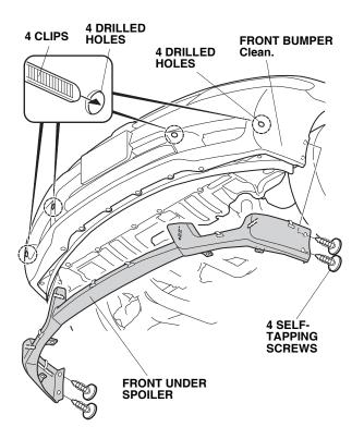
22. Position the front under spoiler on the front bumper, and loosely tighten four self-tapping screws as shown.
