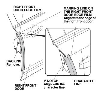
7. While slowly removing the backing on the backside of the right front door edge film, attach the right front door edge film to the right front door securely. Align the marking line on the right front door edge film with the edge of the right front door. 8. Insert the applicator into the soft sleeve.
