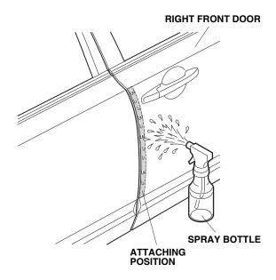
4. Using a spray bottle with 3M protective tape application solution, spray the area where the right front door edge film will attach.
