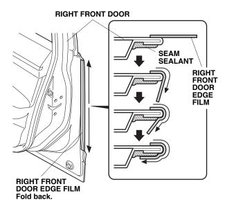
12. Wipe the water from the right front door edge film using a shop towel. Allow the right front door edge film to dry thoroughly.
