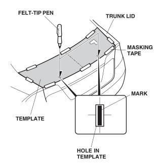
11. Position template A on the trunk lid. Using a felt-tip pen, mark the trunk lid on the left and right sides.
