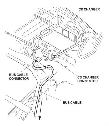
39. Fold the excess bus cable and secure the bus cable to the holes in the rear seat panel with two wire ties with clips.
