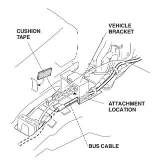
28. Pull back the floor carpet, and attach the bus cable to the floor panel with three cushion tapes in the areas shown.
