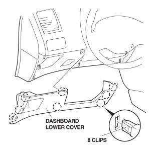
15. Release the four clips, and remove the passenger's dashboard under cover by pulling it toward you. Take care not to damage the clips and pins.
