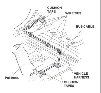
29. Secure the bus cable to the vehicle harness with five wire ties in the areas shown.
