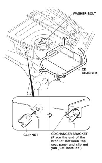
37. Slide two clip nuts onto the CD changer bracket and rear shelf through the holes in the parcel shelf, and align their holes as shown. Install two washerbolts, and tighten them securely.
