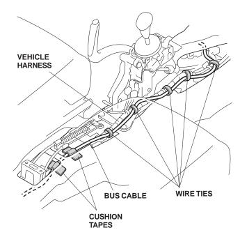
27. Using isopropyl alcohol on a shop towel, clean the area where the cushion tapes will attach. Attach the bus cable to the floor panel with two cushion tapes in the areas shown.
