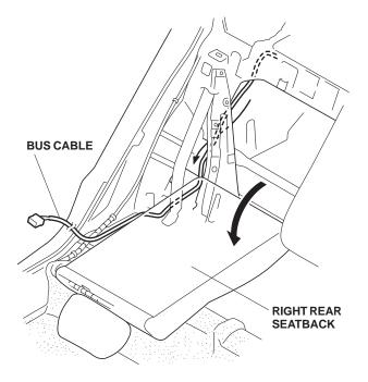
21. Lift up the right rear seatback, then remove the clip securing the floor carpet. Turn over the floor carpet.
