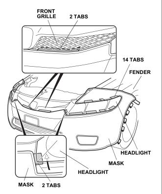
9. Pull the mask toward the wheelwell, smooth out any wrinkles, attach the five plastic hooks to the fenderwell, then bend the metal tab around the fenderwell. Repeat on the other side.
