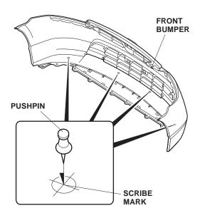
4. While wearing eye protection, drill a 10 mm hole through each marked location from the outside of the bumper. First drill with a 3 mm bit, then finish with a 10 mm bit. Remove any burrs from the edges of the holes with a file.
