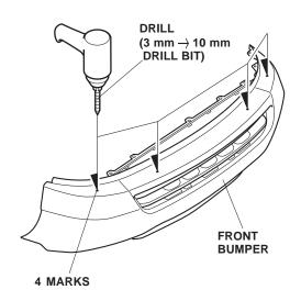
5. While wearing eye protection, drill a 3 mm hole through each of the four dimples on the ends of the front bumper. Remove any burrs from the edges of the holes with a file.
