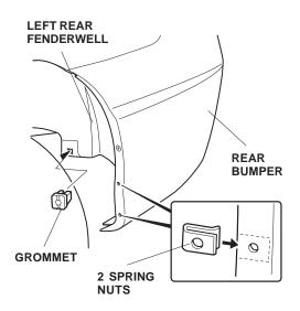
Position the left rear splash guard on the left rear fenderwell and rear bumper, then install the three 5 x 20 mm self-tapping screws. Tighten the three self-tapping screws in the order shown. Cut off any excessive undercoat material with a utility knife.
