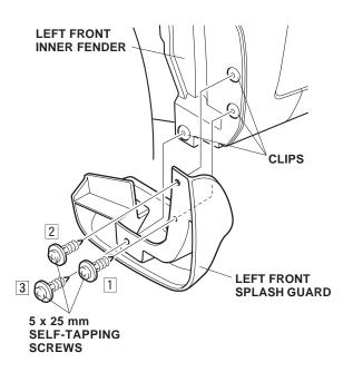
4. Turn the steering wheel all the way clockwise, and repeat steps 2 and 3 to install the right front splash guard.
