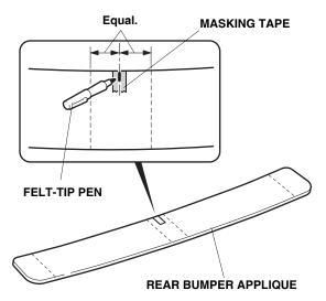
3. Position the rear bumper applique on the rear bumper, then attach masking tape to the rear bumper as shown.
