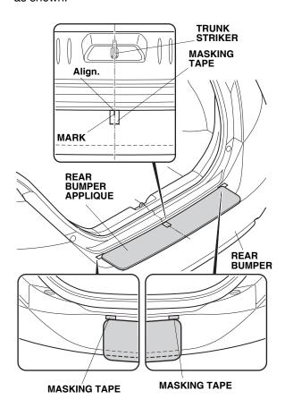
Remove the backing shown. Using the applicator
