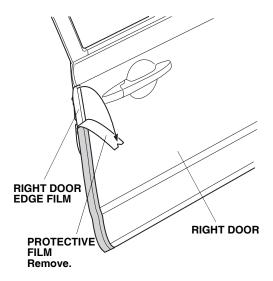
11. Starting from the middle and working outward, fold over the right door edge film onto the inside of the right door as shown. Move your fingers in one direction only.
