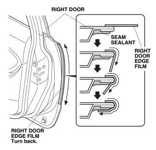
12. Wipe up water from the right door edge film using a shop towel. Allow the right door edge film to dry thoroughly.
