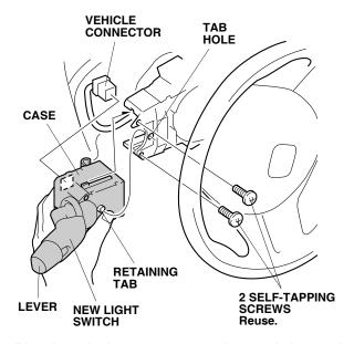
35. Plug the vehicle connector into the new light switch.
