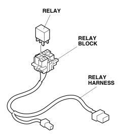
26. Plug the relay harness 8-pin connector into the open 8-pin connector on the fuse box.
