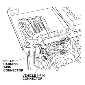
28. Remove lower hood opener bolt, and secure the relay bracket to the vehicle panel with the hood opener bolt.
