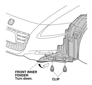
2. Insert your hand inside of the inner fender released in step 1. Unplug the connector from the fog light, and remove the bulb.
