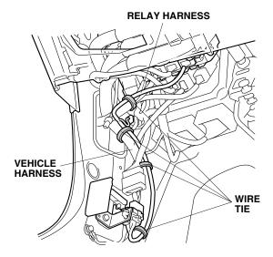
32. Turn the steering wheel counterclockwise. Unplug the vehicle connector, and unplug the vehicle harness from the light switch.
