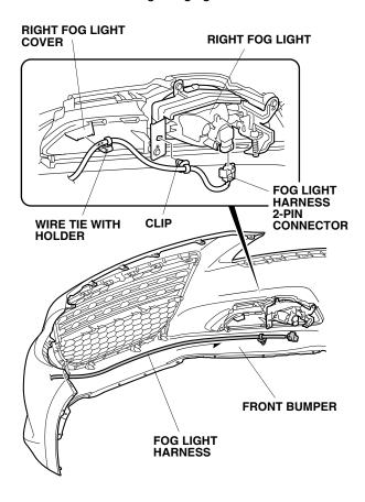
18. Attach wire tie with holder to the right fog light cover, and attach the clip to the right fog light.
