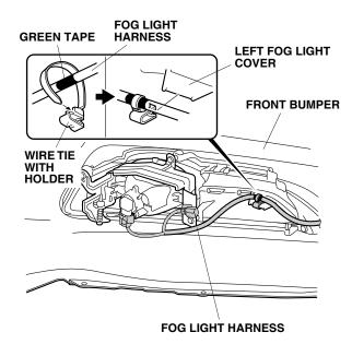
17. Route the other fog light harness 2-pin connector to the right side of the front bumper, and plug the 2-pin connector into the right fog light.
