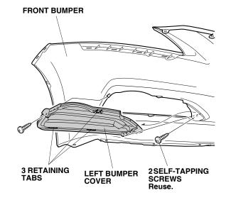
11. Install the left fog light cover to the front bumper with three retaining tabs and one self-tapping screw removed in step 10.
