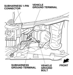
22. Locate the green tape on the subharness. Install the wire tie with clip to the subharness at the green tape. Insert the wire tie with clip into the hole in the vehicle frame.
