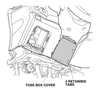
4. Remove the driver's under cover (turn the knob, two clips, and one pin).
