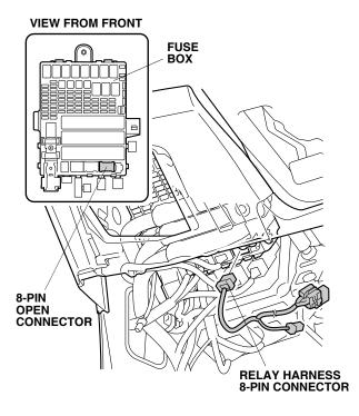
NOTE: If the 8-pin connector is already used by another accessory, locate the 8-pin connector taped to that other accessory harness. Remove the tape and dummy connector from that other accessory harness. Plug the fog light harness 8-pin connector into that other accessory harness.
