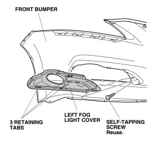
12. Install the left fog light to the front bumper with two 5 x 14 mm self-tapping screws and one self-tapping screw removed in step 10.
