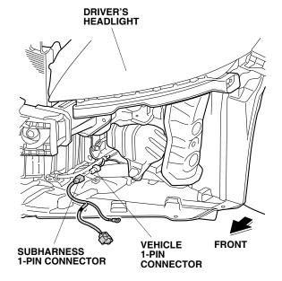
21. Just above the subharness 1-pin connector, locate the vehicle ground bolt. Remove the vehicle ground bolt, and install the ground terminal from the subharness using the vehicle ground bolt.
