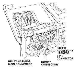
27. Plug the relay harness 1-pin connector into the vehicle 1-pin connector.
