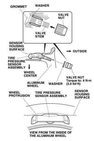
2. Remove the valve cap. Install the tire pressure sensor and the washer to the wheel, and finger-tighten the valve nut. Make sure the pressure sensor is resting on the wheel.
