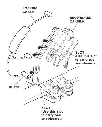
15. After loading each snowboard on to the carrier, adjust it with the help of the board supports so that the top edges are level and the boards are as far down in the carrier as possible. To secure the snowboard, use the key to open the covers, then insert the locking cable stop into the holes of the carrier covers.
