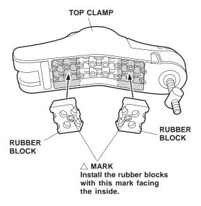
△ MARK Install the rubber blocks with this mark facing the inside.
