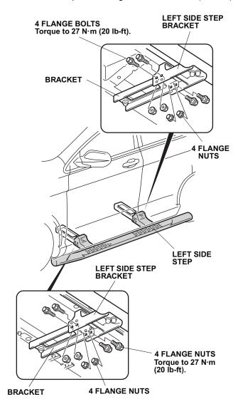
Install the left side step brackets to the vehicle frame using two flange bolts per bracket. Torque the flange bolts to 27 N·m (20 lb-ft). On chrome side steps, torque the four flange bolts at the lower part of the left side step to 27 N·m (20 lb-ft).
