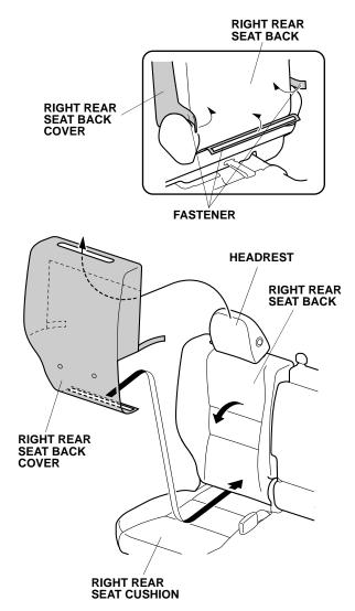
Tilt the right rear seat back forward, and tuck the fastener between the seat back and the seat cushion. Secure the three fasteners to the right rear seat back. 11. Locate the two rubber stops on the front of the right rear seat cushion. Align the two holes in the right rear seat cushion cover over the rubber stops, and install the right rear seat cushion cover over the right rear seat cushion.
