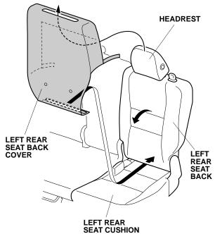
Tilt the left rear seat back forward, and tuck the fastener between the seat back and the seat cushion. Secure the three fasteners to the left rear seat back.  Locate the two rubber stops on the front of the left rear seat cushion. Align the two holes in the left rear seat cushion cover over the rubber stops, and install the left rear seat cushion cover over the left rear seat cushion.
