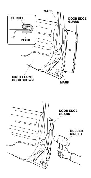
7. Repeat steps 3 thru 6 to install the left front door edge guard.
