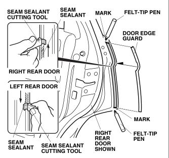
9. Position the cutting edge of the seam sealant cutting tool against the door edge, and trim the seam sealant from mark to mark.
