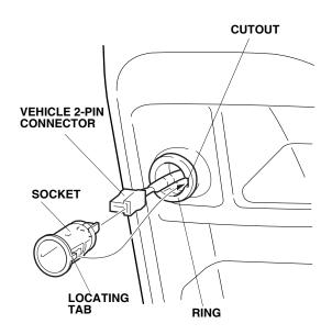
9. Align the locating tab on the socket with the cutout in the ring, and slide the socket into the ring.
