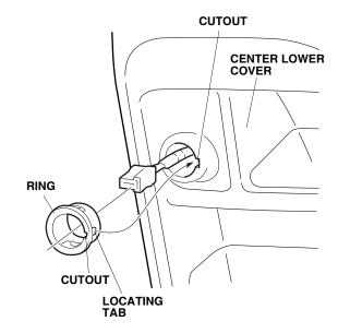
8. Push the vehicle 2-pin connector into the socket.
