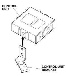
25. Plug the back-up sensor harness 14-pin connector into the control unit.
