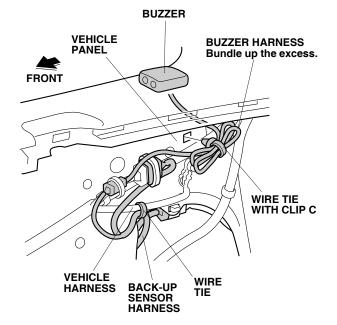
40. Bundle up the excess buzzer harness, and secure it to the vehicle panel with one wire tie with clip C.
