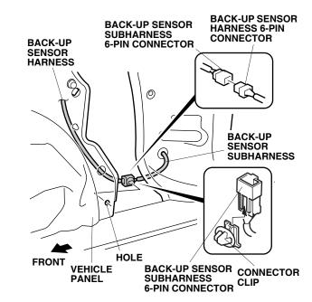
44. Plug the back-up sensor subharness 6-pin connector into the back-up sensor harness 6-pin connector, and install the connector clip. Secure the clip in the vehicle panel hole in the area shown. 45. Route the back-up sensor subharness as shown, and install the back-up sensor subharness clip into the vehicle panel hole.
