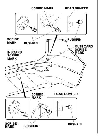
49. Inside the rear bumper on the *passenger's side*, locate the two back-up sensor scribe marks. Using a pushpin, pierce the center and top for both the outboard and the inboard scribe marks. There are several marks on the inside of the rear bumper; make certain that you locate and pierce the proper scribe marks.
