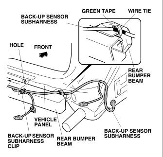
*Without rear bumper beam:* Secure the subharness to the stud on the vehicle panel with one wire tie with clip A at the green tape.
