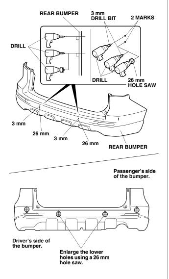
51. Enlarge the lower 3 mm holes using a 26 mm hole saw.
