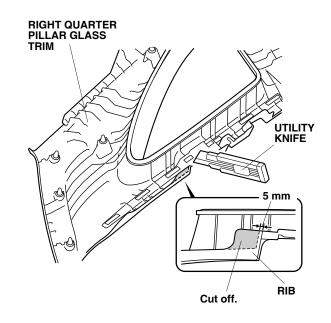
30. Using a scale and a felt-tip pen, measure and mark the right quarter pillar glass trim in the area shown.
