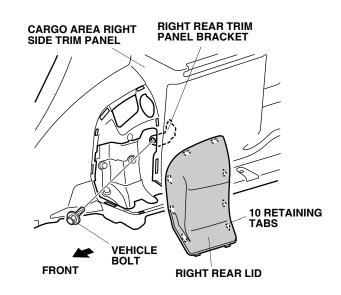
8. Remove the vehicle bolt from the right rear trim panel bracket.
