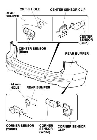
55. On the *driver's side* of the rear bumper, install the corner sensor (white) and the center sensor (blue) to the rear bumper using one corner sensor clip, and one center sensor clip. Be sure the sensors are seated properly.
