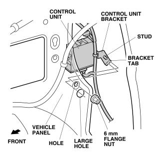
28. Install the back-up sensor harness clip into the hole in the vehicle panel.
