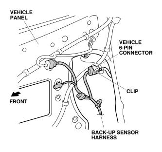
22. Wrap one EPT sealer around the back-up sensor harness 6-pin connector, and secure the 6-pin connector to the vehicle harness with one wire tie.
