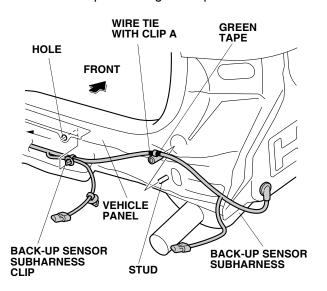
46. Route the back-up sensor subharness as shown. Install the back-up sensor subharness clips into the holes in the vehicle panel.
