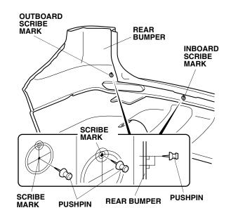
50. While wearing eye protection, drill a 3 mm hole at each of four pierced points you made in the center of the rear bumper.
