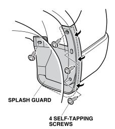
14. Remove the right rear splash guard (four self-tapping screws).
