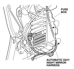
18. Remove the steel wire. Route the automatic day/ night mirror harness along the vehicle harness as shown. Loosely secure the day/night mirror harness to the vehicle harness with four wire ties.
