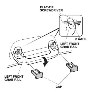
10. Using needle nose pliers, remove the left front grab rail (two clips).
