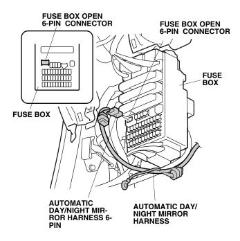
NOTE: If another accessory is already plugged into the 6-pin connector opening of the fuse box, remove the dummy connector from the 6-pin connector taped to the automatic day/night mirror harness. Plug the 6-pin connector from the other accessory harness into the 6-pin connector on the automatic day/night mirror harness and plug the automatic day/night mirror harness into the 6-pin connector opening of the fuse box.
