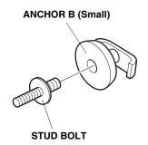
55. Attach a spacer and stud bolt to an anchor B (Small). NOTE: The direction of the spacer.
