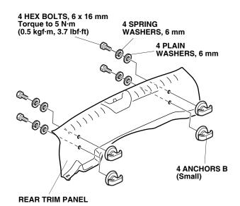
29. Reinstall the rear trim panel (four clips and three hooks).
