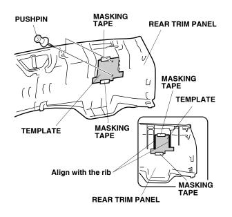
27. While wearing eye protection, drill a 3 mm hole at the four marked points, then finish with a 6.5 mm bit. Remove any burrs from the edge of the holes using a round file.
