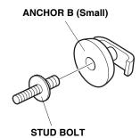
18. Attach a spacer and a stud bolt to an anchor B (Small).
