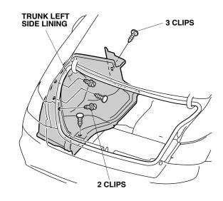
4. Remove the trunk right side lining the same way.
