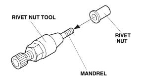
Insert the rivet nut into the hole in the trunk left side panel and install the hex wrench on the rivet nut tool.
