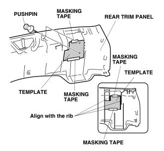
64. While wearing eye protection, drill a 3 mm hole at the four marked points, then finish with a 6.5 mm bit. Remove any burrs from the edge of the holes using a round file.
