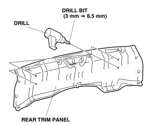
65. Install the four anchors B (Small) to the rear trim panel with four 6 x 16 mm hex bolts, four 6 mm spring washers, and four 6 mm plain washers as shown. Torque the 6 x 16 mm hex bolts to 5 N·m (0.5 kgf·m, 3.7 lbf·ft). Position the anchors as shown.
