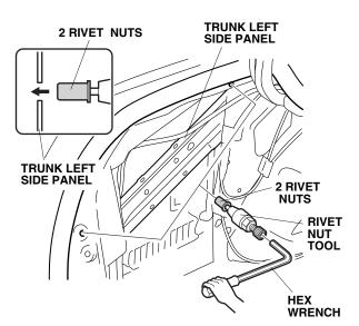
41. While holding the rivet tool with the hex wrench, turn the 27 mm wrench clockwise and install the rivet nut to the left trunk side panel.
