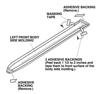
5. Align the end of the left front body side molding with the front template as shown and attach it at the front and back.
