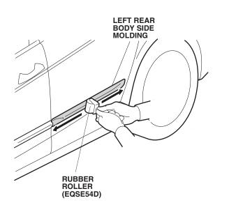
14. Turn the templates over and repeat steps 1 thru 13 to install the body side molding on the right side of the vehicle.
