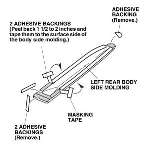
10. Align the end of the left rear body side molding with the rear template as shown and attach it at the front and back.
