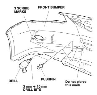
While wearing eye protection, drill the three pierced marks on the front bumper with a 3 mm drill bit, then enlarge the holes with a 10 mm drill bit. Remove any burrs. 11. Drill two holes at the two dimples in the front bumper with a 5 mm drill bit. Remove any burrs.
