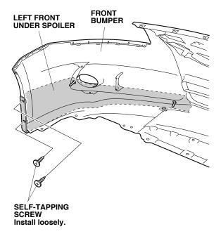
18. Secure the left front under spoiler to the front bumper with two clip retainers and four seals. Using diagonal cutters, cut the excess off the two clips as shown.
