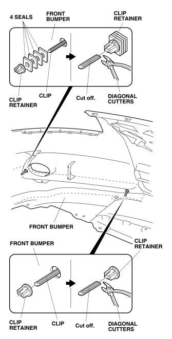
19. Secure the left front under spoiler to the front bumper with one clip.
