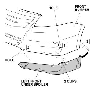
17. Loosely install two self-tapping screws to the left front under spoiler and bumper.
