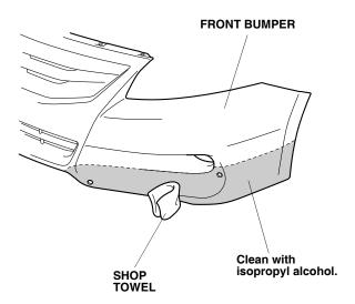
16. Install the left front under spoiler to the front bumper in the order shown.
