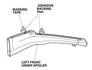
15. Using isopropyl alcohol on a shop towel, thoroughly clean the area where the left front under spoiler will attach.
