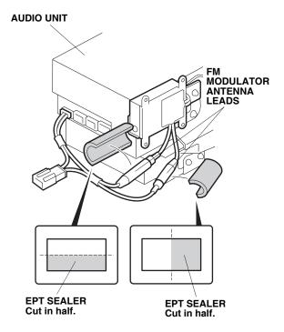
116. Plug the vehicle antenna connector to the subfeeder antenna 2-pin connector.
