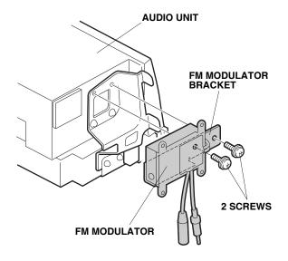
114. Plug the sub-feeder antenna leads to the FM modulator antenna leads. Plug the sub-feeder 2-pin connector into the audio unit.
