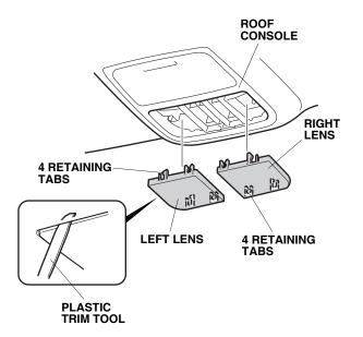
4. Open the console pocket lid, and remove the roof console (four bolts and unplug the vehicle connectors).
