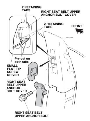
23. Remove the right seat belt upper anchor bolt.
