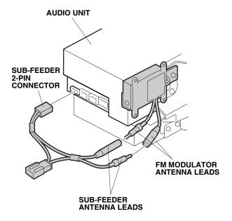
115. Using scissors, cut two EPT sealers in half as shown. Wrap two pieces of EPT sealers around the FM modulator antenna leads as shown.
