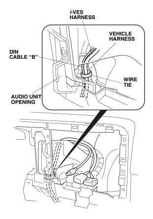
87. Plug the *i*-VES harness 20-pin connector into the vehicle 20-pin connector, and secure the 20-pin connectors with one long wire tie.
