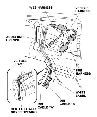
55. Align the sub harness 24-pin connector and the DIN cable "B" connector to the vehicle 24-pin connector, and secure them to the vehicle harness with two wire ties.
