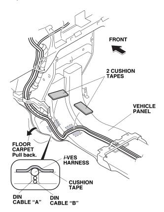
85. Secure the *i*-VES harness and the DIN cables to the vehicle harness with two wire ties.
