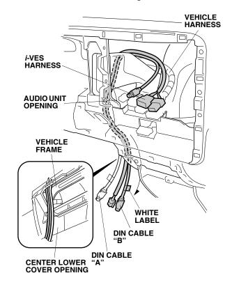
51. Route the *i*-VES harness, DIN cable "A" and DIN cable "B" to the rear of the vehicle. Go to step 60.
