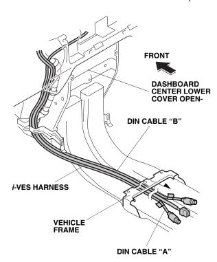
52. Wrap one urethane tape to the *i*-VES harness 20-pin connector and the *i*-VES harness as shown.
