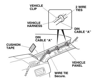
95. Secure the DIN cable "A" to the vehicle harness with two wire ties, and secure the wire tie loosely secured in step 45.
