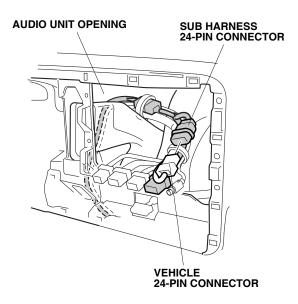
57. Secure the *i*-VES harness and the DIN cable "B" to the vehicle harness with one wire tie.
