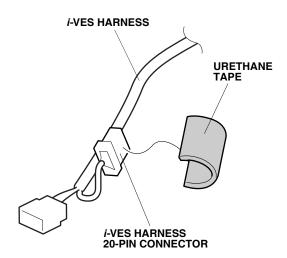
53. Plug the sub harness 20-pin connector into the *i*-VES harness 20-pin connector.
