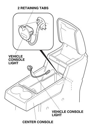
38. Remove the center console (two bolts and two self-tapping screws).
