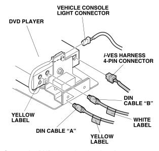
80. Secure the DVD player bracket A to the center console with two 5 mm stepped bolts and two 5 mm cap nuts.
