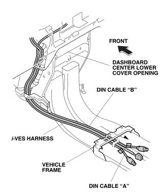
59. Secure the *i*-VES harness and the DIN cables to the vehicle harness with one wire tie.
