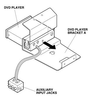
73. Secure the auxiliary input jacks to the DVD player bracket B with two 3 x 8 mm screws and two 3 mm nuts.
