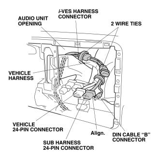
56. Plug the sub harness 24-pin connector to the vehicle 24-pin connector.
