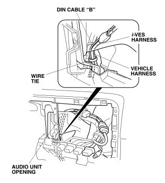
58. Route the *i*-VES harness, DIN cable "A" and DIN cable "B" to the rear of the vehicle.
