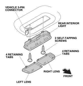
97. Remove the rear interior light (two self-tapping screws and unplug the vehicle 3-pin connector).
