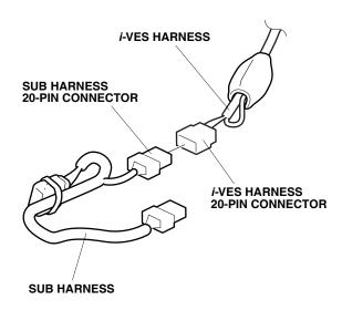
54. At the audio unit opening, route the *i*-VES harness and the white label side of the DIN cable "B" from the audio unit opening down towards the vehicle floor along the vehicle harness.
