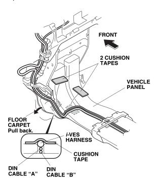
90. Secure the *i*-VES harness and the DIN cables to the vehicle harness with two wire ties.
