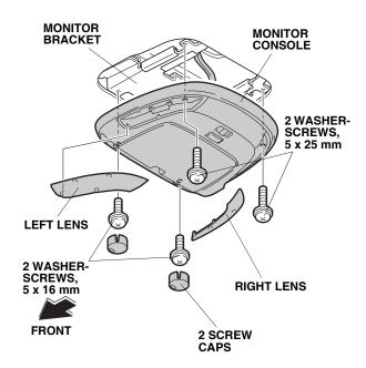
109. Install two screw caps, then reinstall the left and right lenses.
