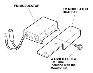
111. Set the FM modulator switch at 88.5. Using isopropyl alcohol on a shop towel, clean the area where the EPT sealer will attach. Using scissors, cut one EPT sealer in half. Secure the FM modulator cables to the FM modulator with one piece of EPT sealer.
