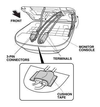
108. Position the monitor console on the monitor bracket, and install the monitor console to the monitor bracket with two 5 x 16 mm washer-screws and two 5 x 25 mm washer-screws. Do not pinch the DIN cable "A" between the monitor console and the monitor bracket.
