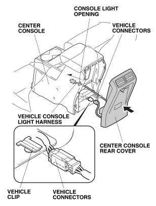
71. Route the vehicle console light harness through the console light opening, and reinstall the center console rear cover.
