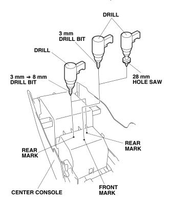
68. Using a 28 mm hole saw, widen the front mark. Remove any burrs.
