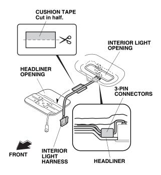
101. Position the 3-pin connectors in the cavity in the headliner. Reinstall the rear interior light.
