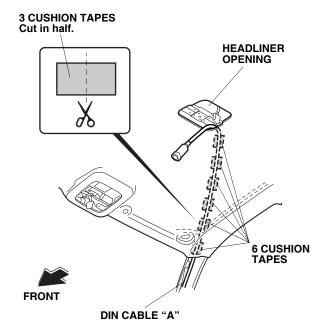
103. Using isopropyl alcohol on a shop towel, clean the areas where the EPT sealers will attach. Using a scissors, cut three EPT sealers in half. Attach six pieces of EPT sealers to the monitor bracket in the areas shown. Cut off the excess of the EPT sealers.
