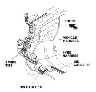
91. Bundle the excess *i*-VES harness, and secure it to the vehicle harness with one long wire tie.
