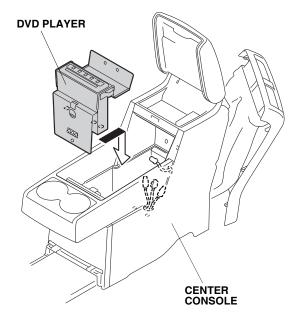
79. Plug the *i*-VES harness 4-pin connector, DIN cable "A", DIN cable "B", and the vehicle console light connector to the DVD player. Do not interchange the connection point of the DIN cable "A" and DIN cable "B"
