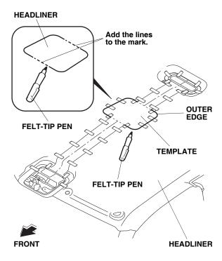
42. Using a utility knife, cut out the marked area of the headliner, and cut out the insulator from the vehicle frame as shown.
