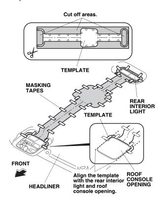
40. Position the template on the headliner and align the cutout with the rear interior light and roof console opening. Tape the template to the headliner with the masking tapes.
