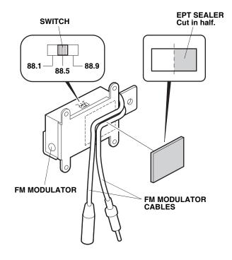
112. Using isopropyl alcohol on a shop towel, clean the area where the EPT sealer will attach. Attach one half EPT sealer cut in step 111 to the audio unit.
