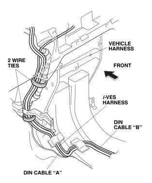
86. At the audio unit opening, secure the *i*-VES harness and the DIN cable "B" to the vehicle harness with one wire tie.
