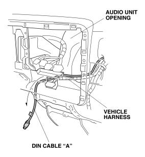
If the vehicle connector at the audio unit opening is 20-pin, continue with step 50; if the vehicle connector is 24-pin, go to step 52.
