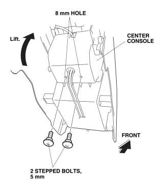
82. Using an isopropyl alcohol on a shop towel, clean the areas where the cushion tapes will attach. Lift the center console, and secure the *i*-VES harness and the DIN cables to the vehicle panel with two cushion tapes.
