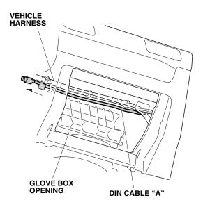
49. Route the DIN cable "A" to the audio unit opening down towards the vehicle floor.
