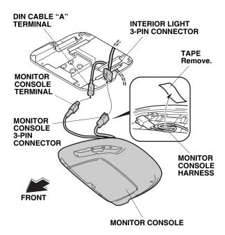
107. Using isopropyl alcohol on a shop towel, clean the area where the cushion tape will attach. While holding the monitor console, secure the 3-pin connectors and the terminals to the monitor console with one cushion tape.
