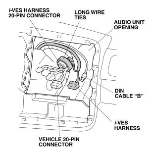
88. Secure the *i*-VES harness and the DIN cable "B" to the vehicle harness with two wire ties. Go to step 92.
