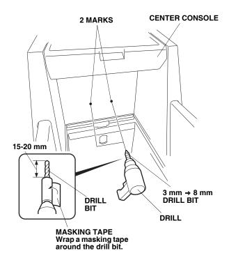
64. While wearing eye protection, drill an 8 mm hole at each marked point. Start with a 3 mm drill bit and finish with an 8 mm drill bit. Remove any burrs.
