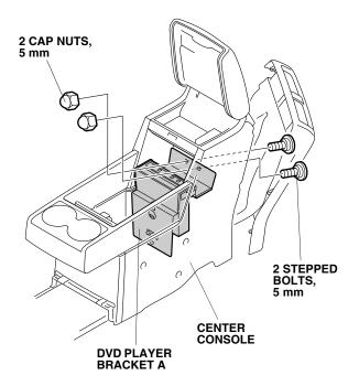
81. Lift the center console as shown, and secure the DVD player bracket A to the center console with two 5 mm stepped bolts.
