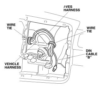
89. Pull back the floor carpet. Using isopropyl alcohol on a shop towel, clean the areas where the cushion tapes will attach. Secure the *i*-VES harness and the DIN cables to the vehicle panel with two cushion tapes.
