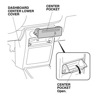
32. Remove the dashboard center lower cover (three self-tapping screws, five clips, six retaining tabs, and unplug the vehicle connectors).
