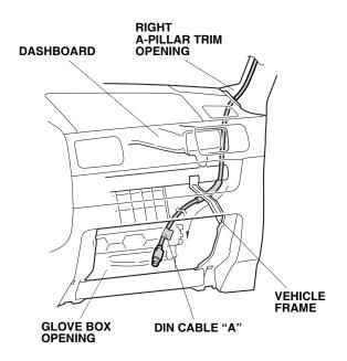
48. Inside the glove box opening, route the DIN cable "A" along the vehicle harness and towards the driver side of the vehicle.
