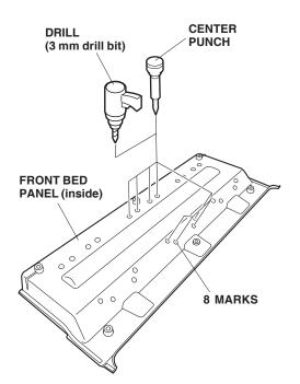
4. While wearing eye protection, enlarge the eight holes to 9 mm from the outer surface side of the front bed panel. Remove all burrs from the edges of the holes with a file.
